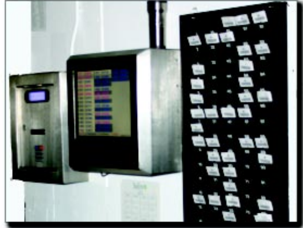
The car request display is one of the key components of the system. The ticket reader instantly alerts the valet when a car is requested and displays when a valet has responded to the request.
